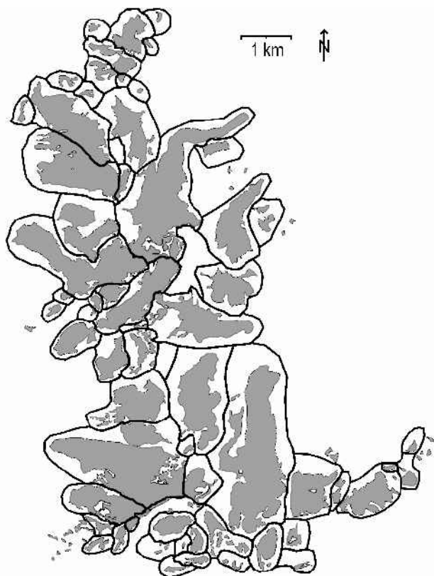
Fig. 5. Glacier basins (bold black lines) and the digitized Swiss glacier inventory of 1973 (grey areas). Contiguous ice masses were separated into individual glaciers according to the 1973 inventory, and roughly surrounded to obtain closed polygons. These polygonal glacier basins can also be used to eliminate gross classification errors (e.g. proglacial lakes) and for glacier identification, especially to assign a unique ID to glaciers.
